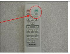
Point the data projector remote at the data projector and press the "Input 1" button.
