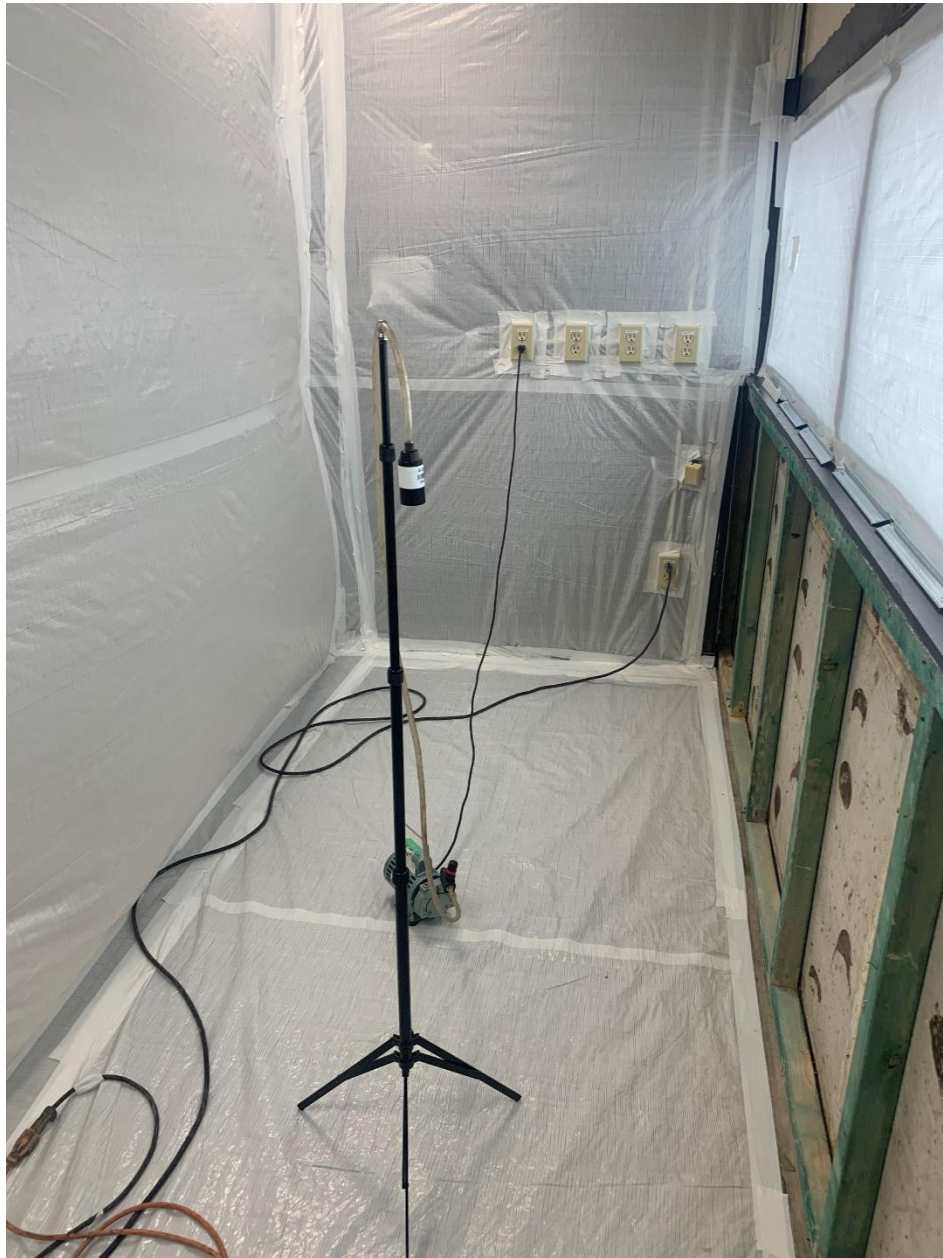
Photograph 1: View of asbestos air sampling within the enclosure of room B2 120.
